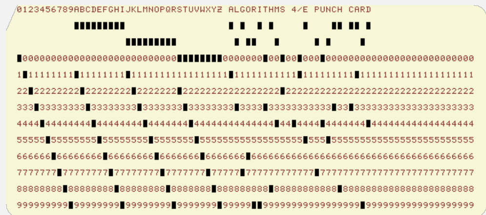
punch card (12 holes per column)
